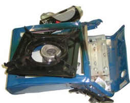
Image 2: A portable gas stove with integrated cylinder that has overheated and exploded.
